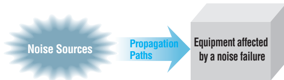
Figure 1.5.1 Overview of Noise Generation and Propagation Path
